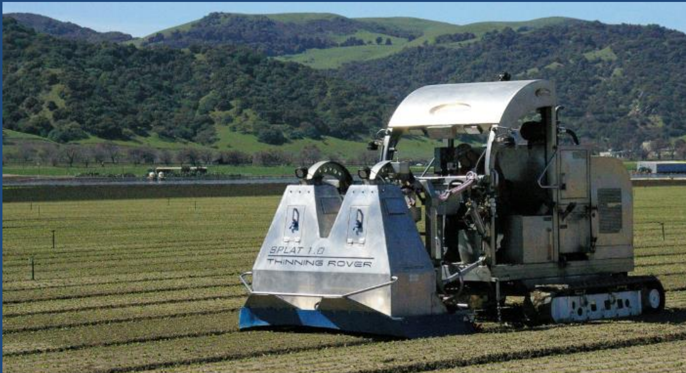
A lettuce thinner created by an agricultural tech startup uses cameras and sensors to thin lettuce rows. Salinas, Calif., has hired a venture capital fund to help it attract other high-tech agricultural companies to the area.
